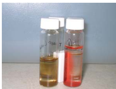
Figure 1. CoSe nanoparticles (brown) and CrSe nanoparticles (red) in an aqueous solution. The nanoparticles are accumulating to one side of the vial, close to the white magnet (center) – demonstrating that they are influenced by a magnetic field.
