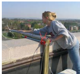
Figure 4. Christy Kull adjusts the flux measurement system on top of the roof of Durham Hall.
